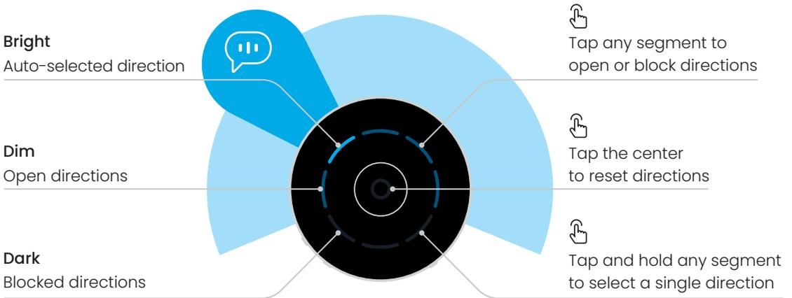
**Device orientation:** open segments face the group, blocked segments face you
